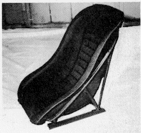
Anatomic racing seat. Steel tube supported plastic shell. Covered in matte black nap. From 33, used in GTA, GTA Jr., GTAm
